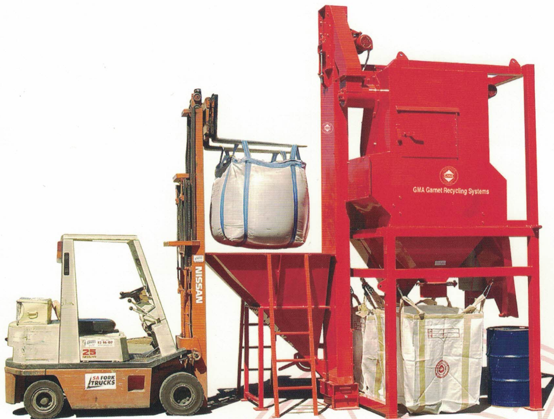
A 2.5 tonne forklift is ideal for continual loading and unloading of Garnet from the recycling unit.
